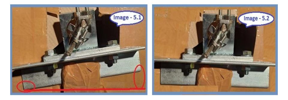
On both side of the belt cleaner, the angle bracket should be welded horizontally straight as shown in Image 5.2
