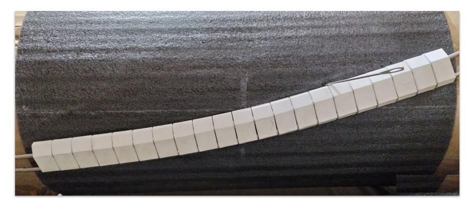
If the metal part/rod is travelling with conveying material and get in contact with the belt cleaner, it may get stuck at the cleaning point. This can lead to tear the rubber belt and damage the belt cleaner.
