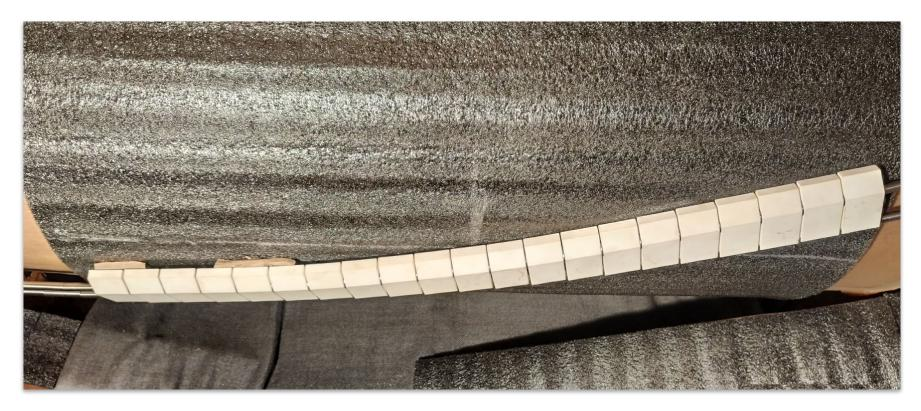
Due to the less tension the foreign particle may get stuck in between the belt cleaner and belt surface. This can lead to twisted belt or material spillage. To prevent this inspect the belt surface and check the spring tension periodically.
