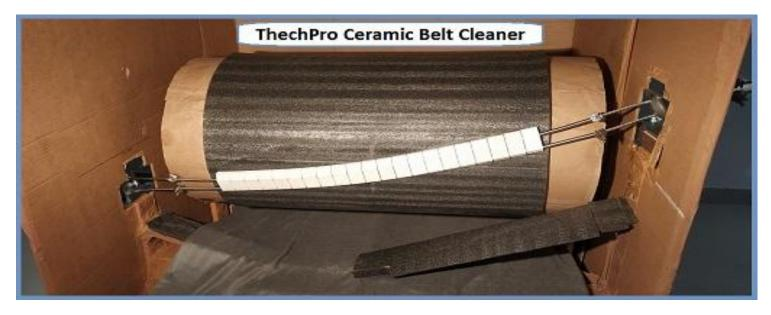
Draw a straight line considering head pulley center point, taking this line reference draw a straight line on belt. This will become center line of head pulley.
